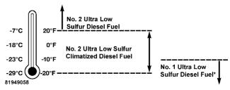
\*No. 1 Ultra Low Sulfur diesel fuel should only be used where extended arctic conditions (-10°F/-23°C) exist.
